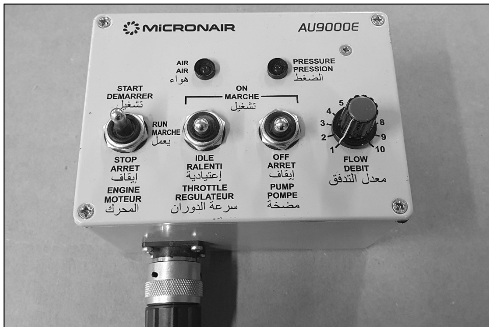
Fig. 1 – Control Box in Cab of Vehicle
