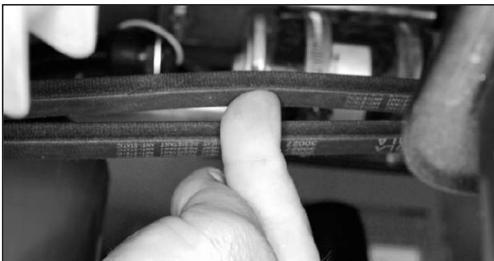
Fig. 8 – Belt Tension Check
