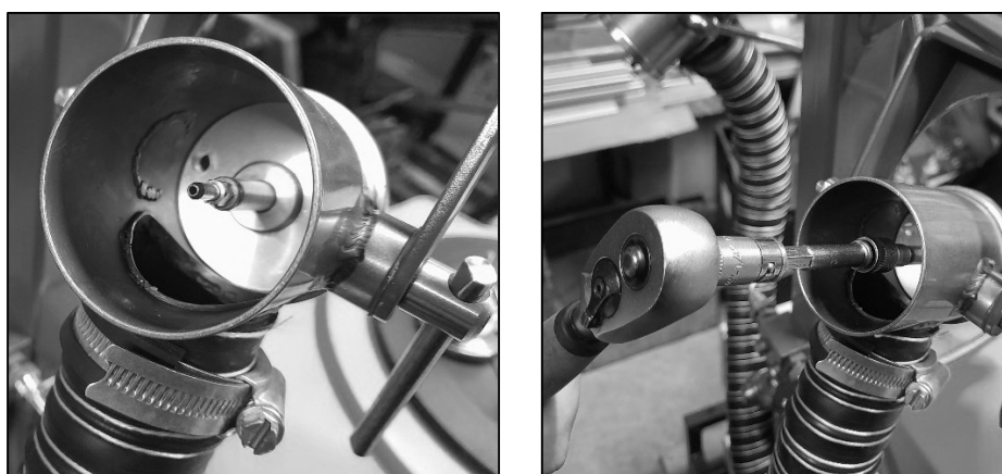
Fig. 13 – Removal of Atomiser Feed Nozzle
