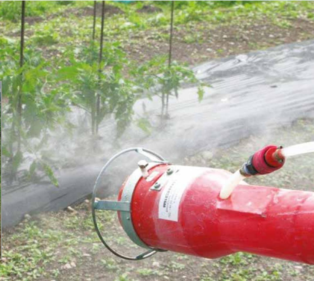
The Micronex rotary atomiser attachment allows most motorised mistblowers to be converted for low and ultra low volume (ULV) spraying to improve spray coverage and increase productivity. The Micronex attachment is particularly suitable for ULV application to control migrant pests such as locusts, as well as flies and mosquitoes. The Micronex attachment can also be used for low volume applications to control pests in horticultural crops, vineyards, fruit trees and plantations.
