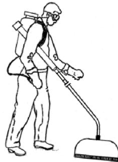
Place the backpack tank on the operator's back and connect to the HANDYDOME
