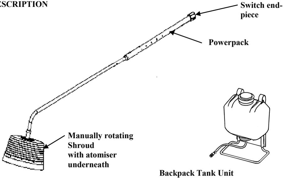
The HANDYDOME is a hand-held, shrouded, spinning disc, Controlled Droplet Application (CDA) sprayer. The HANDYDOME is powered by four ‘torch’ type batteries (D-cell/R20), with one set of good quality batteries giving around 40 hours spraying time. It is designed to apply herbicides, within a manually rotating, 35cm diameter shroud, at volumes of around 50 litres/hectare.
