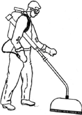
Start walking immediately spray liquid is emitted. When spraying, the spray head should be held as close to the ground or the top of the weed canopy as possible with the shroud at an angle of approx. 5 degrees to the horizontal. The leading edge of the fringe fitted to the shroud should be touching the ground or the top of the weed canopy. The shroud will be seen to rotate. **It is important to rotate the shroud as much as possible in order for the inbuilt Weedswiper to take effect.**
