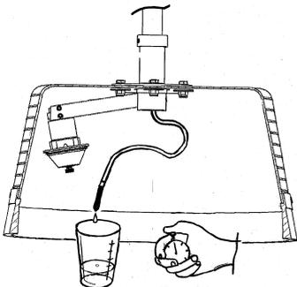
The actual flow rate should be checked holding the HANDYDOME in the spraying position (see 'TO START SPRAYING'). Remove the feed nozzle from the atomiser and allow the liquid to flow into a suitable container .
