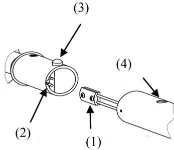
Remove the switch end piece as follows; by unscrewing the Screw Switch Plug
