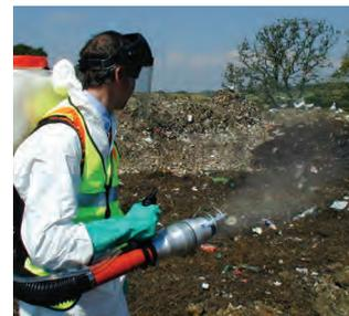
As well as being supplied as part of a complete sprayer, the Micron AU8000 spray head is also available as a conversion kit for suitable mistblowers. The kit includes connecting tubes, handle/control valve, restrictors and all attachments needed to replace a standard mistblower outlet. This kit is suitable for most types of 5HP knapsack mistblowers meeting the air flow requirements given in the specification table.
