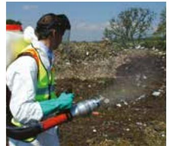
As well as being supplied as part of a complete sprayer, the Micron AU8000 spray head is also available as a conversion kit for suitable mistblowers. The kit includes connecting tubes, handle/control valve, restrictors and all attachments needed to replace a standard mistblower outlet. This kit is suitable for most types of 5HP knapsack mistblowers meeting the air flow requirements given in the specification table.
