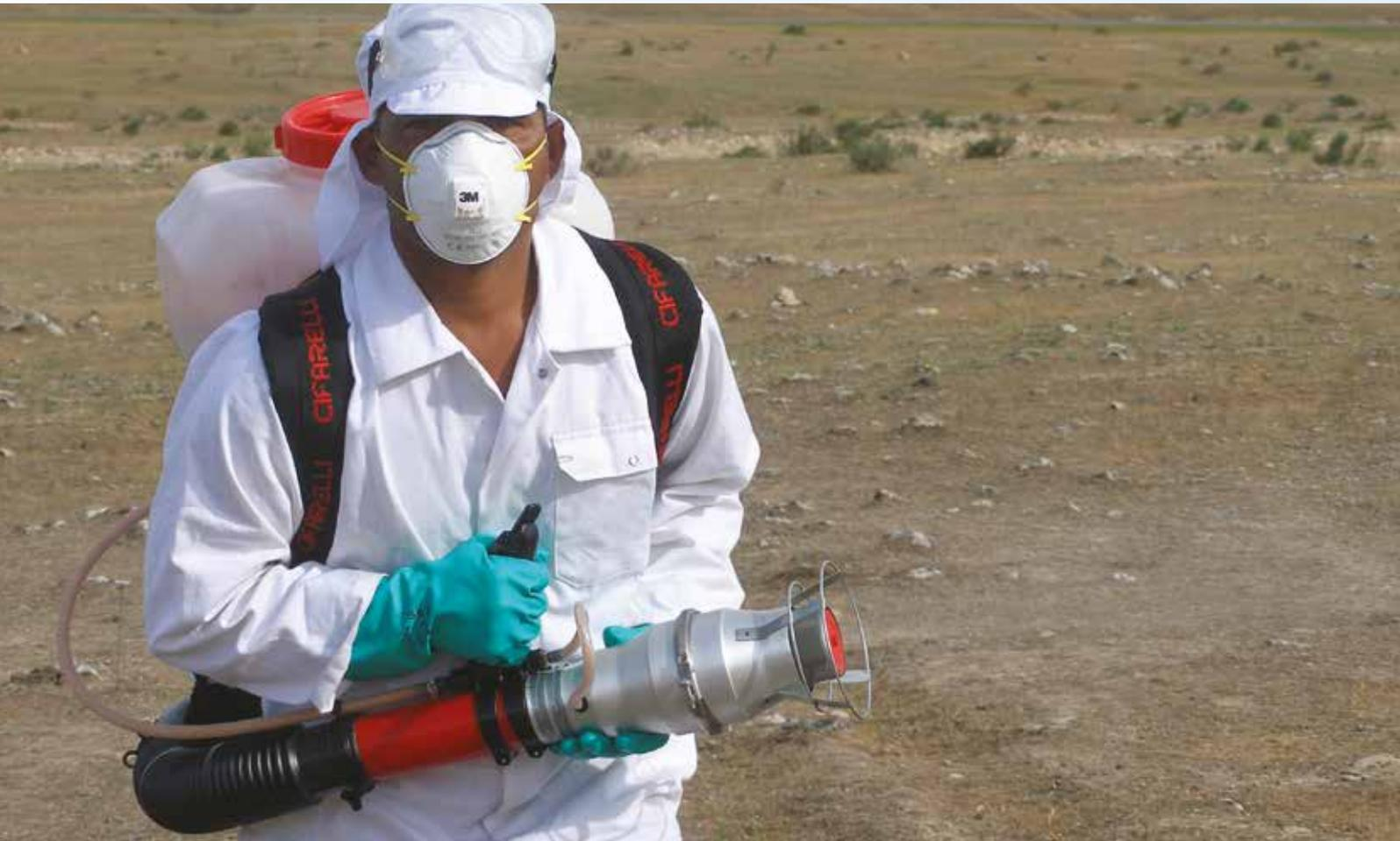
The Micron AU8000 sprayer is a highly efficient knapsack mistblower which brings the advantages of rotary atomiser technology originally developed for agricultural aircraft to ground spraying applications.
