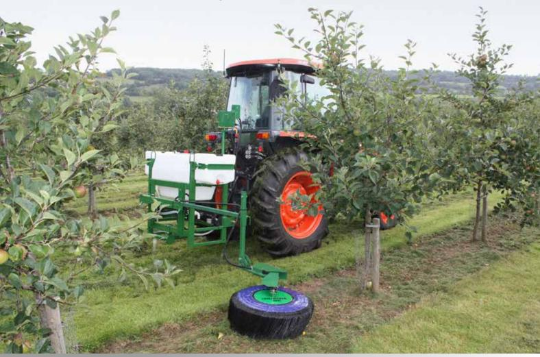
Incorporating either traditional hydraulic pressure nozzles (HiFlo models) or Micron CDA (Controlled Droplet Application) atomisers, the Undavina range of vehicle-mounted sprayers offers an efficient and targeted method of weed control round the base of vines and fruit trees.
