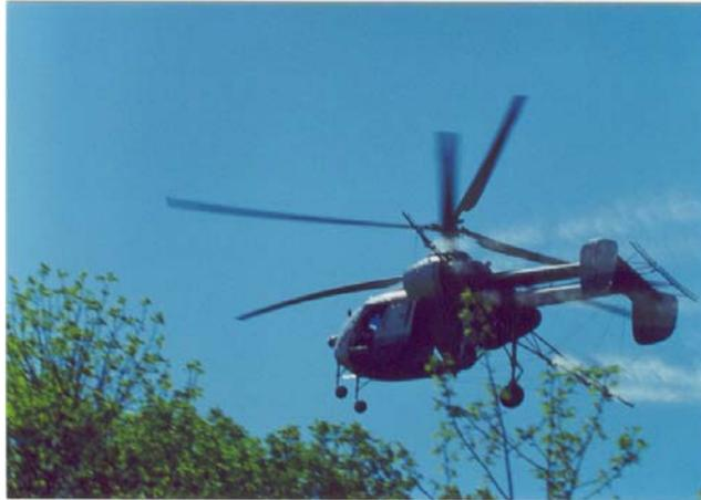
*Kamov K-126 Helicopter with Micronair AU6539 electric atomisers in Eastern Europe*
