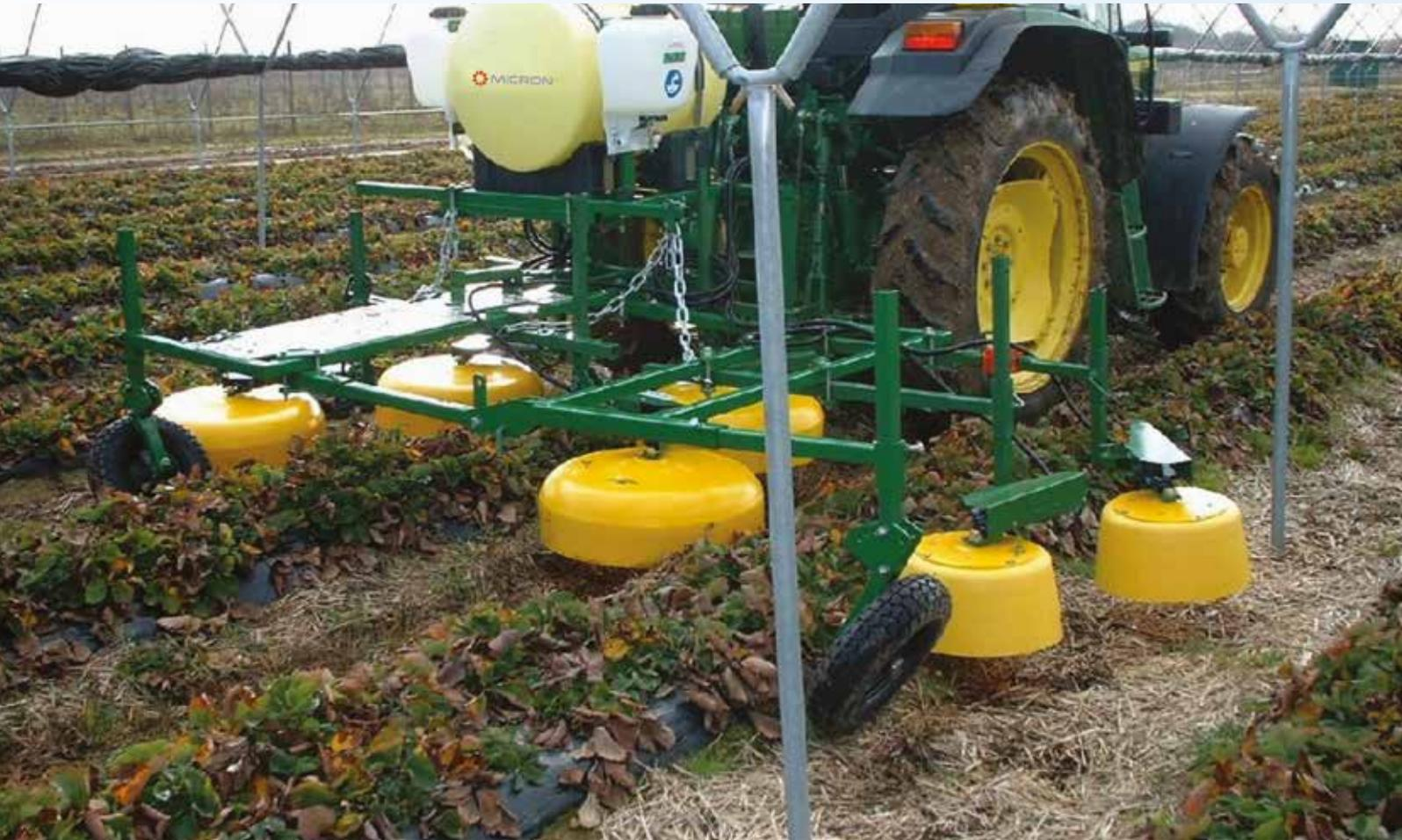
Flexidome is a shielded, tractor-mounted sprayer for weed control in soft fruit grown in raised beds outdoors or in Spanish tunnels.
