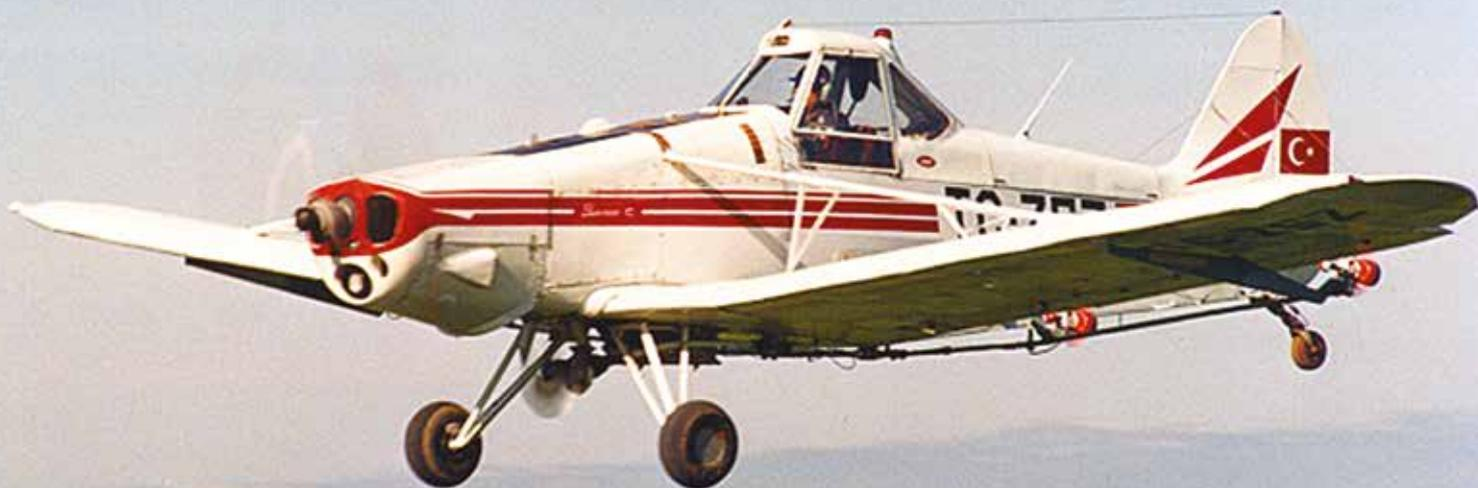
The AU4000 is a precision engineered rotary atomiser designed specifically for use on agricultural aircraft for specialised ultra low volume (ULV) spraying operations. The large diameter gauze assembly and durable bearings are designed for continuous operation at the high rotational speeds required to produce the small droplets necessary for environmental health, migrant pest, forestry and similar ULV spray applications.
